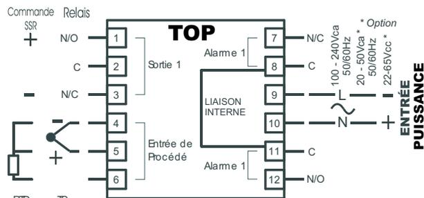
UTILISER DES CONDUCTEURS EN CUIVRE (SAUF POUR ENTREE THERMOCOUPLE)
