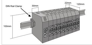
**NOTE:** An additional 60mm of space is required above and below the system modules to permit ventilation and to accommodate wiring bend radii to enclosure trunking or conduits. Allow sufficient slack in all cables inside the trunking to permit "hot" swapping of modules (i.e. modules to be removed/replaced whilst the system is under power).
