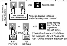
NOTE: Pre-Tune will not engage (a) if the setpoint is ramping, (b) if the process variable is within 5% of input span of the setpoint, (c) if the proportional band = 0 or (d) if Soft Start is operating. It is a single-shot routine and is thus self-disengaging. If PPE = 1 (Auto Pre-Tune enabled - see SET UP MODE), Pre-Tune will run for every power-up.
