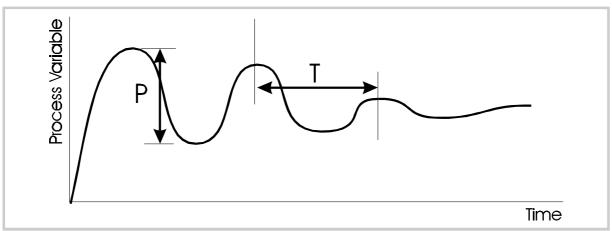
Figure 3-4 Manual Tuning Parameters (Output 1 only)
