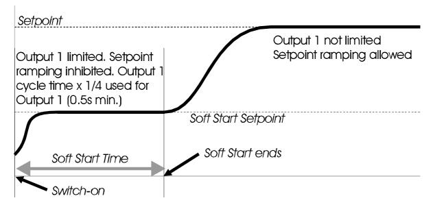
Soft Start Time, Soft Start Setpoint and power limit are all adjustable in Set Up Mode (see Section 3). Soft Start is aborted at start-up if the process variable exceeds the Soft Start Setpoint. Setpoint ramping is inhibited during Soft Start. During a Soft Start, the Soft Start time remaining at any moment may be read from the front panel.
