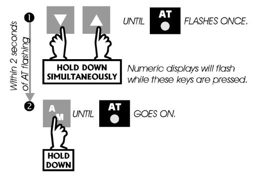
To dis-engage Self-Tune, repeat this procedure (the AT indicator will go OFF).
