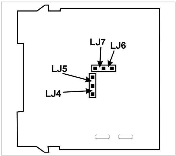
Figure 2-5 PSU PCB Link Jumpers -  $\frac{1}{8}$ -DIN Controllers
