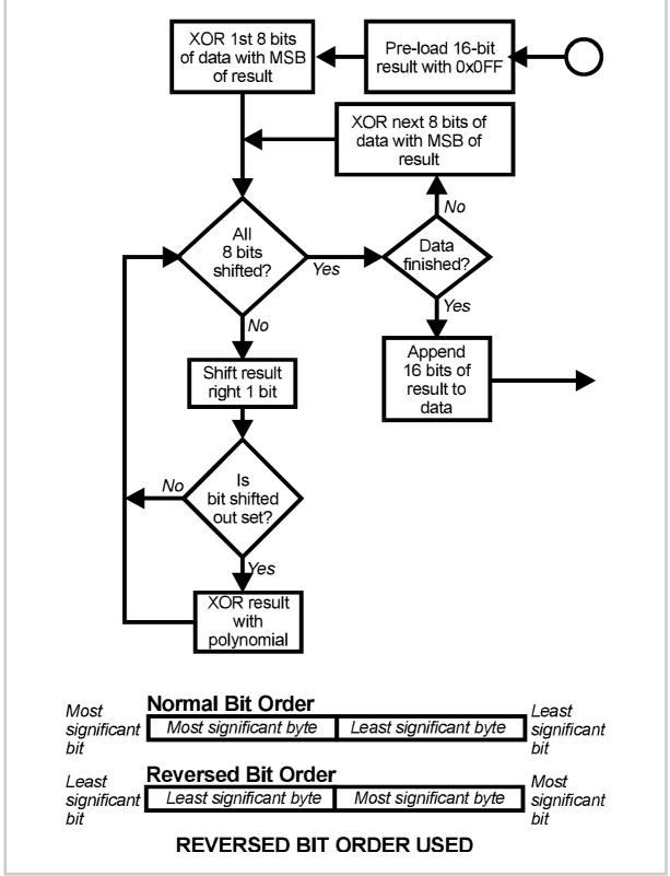
Figure 4-1 Cyclic Redundancy Check Algorithm
