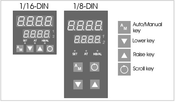
Figure 2-1 Front Panel Indicators and Control Keys
