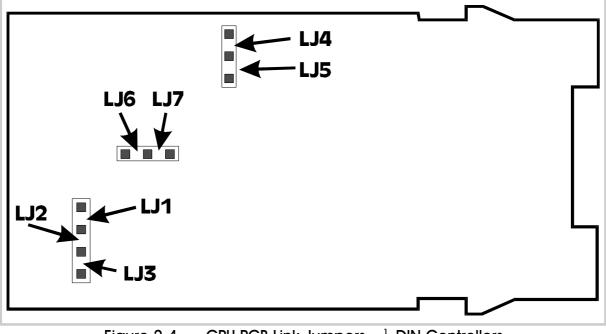
Figure 2-4 CPU PCB Link Jumpers - 1/16-DIN Controllers
