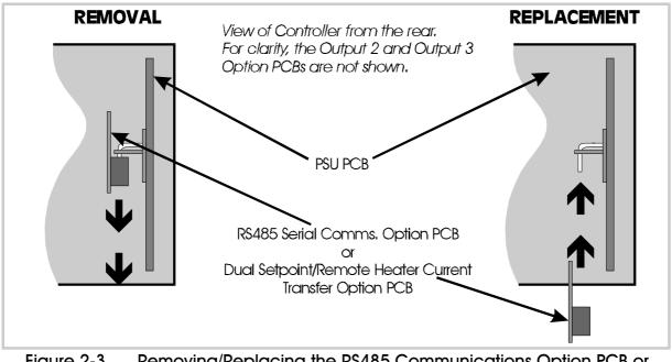
Figure 2-3 Removing/Replacing the RS485 Communications Option PCB or Dual Setpoint/Remote Heater Current Transfer Option PCB
