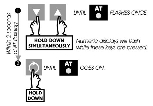
The AT indicator will flash whilst Pre-Tune is operating. To dis-engage Pre-Tune, repeat this procedure (the AT indicator will go OFF).
