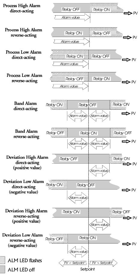
Figure 3-2 Alarm Operation
