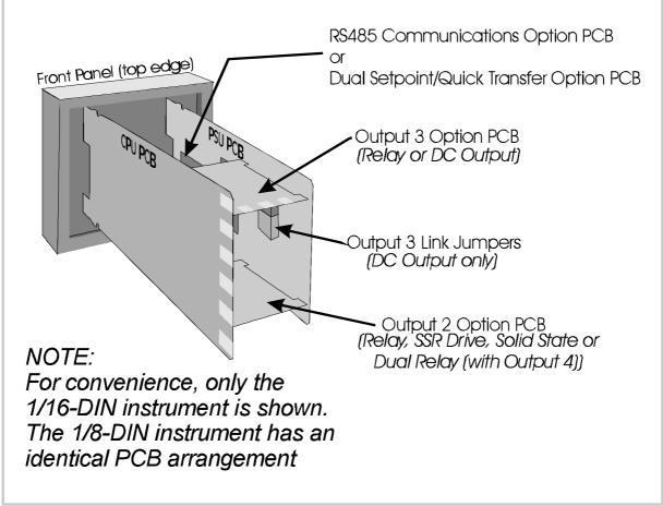
Figure 2-1 PCB Positions
