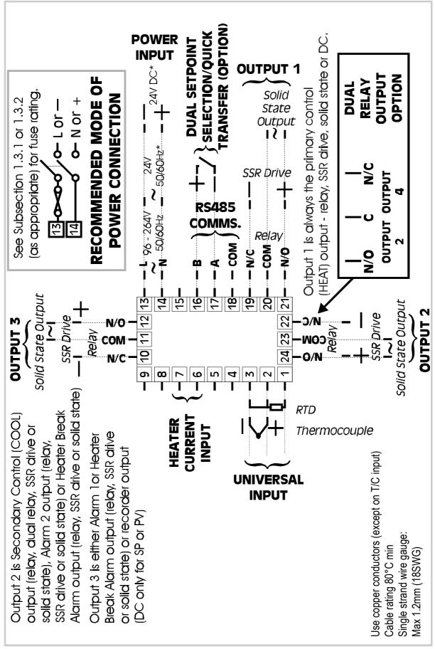
Figure 1-5 Rear Terminal Connections (<sup>1</sup>/<sub>8</sub>-DIN Controllers)
