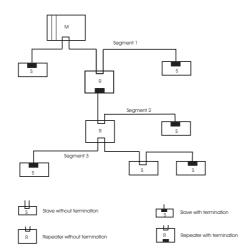
PROFIBUS systems are build as line structure. A PROFIBUS project can be extended by of connection of repeaters,
