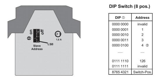
The positions of the switches are shown in binary-code. The number at the lowest position corresponds to the LSB (DIP-switch-position 1). The upper number corresponds to the MSB(DIP-switch-position 8).
