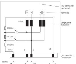
Construction of bus termination
