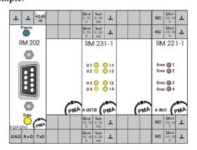
The sketched unit of 5 modules has 4 analog outputs and 4 analog inputs. The user parameterizes the analog I/Os as follows:
